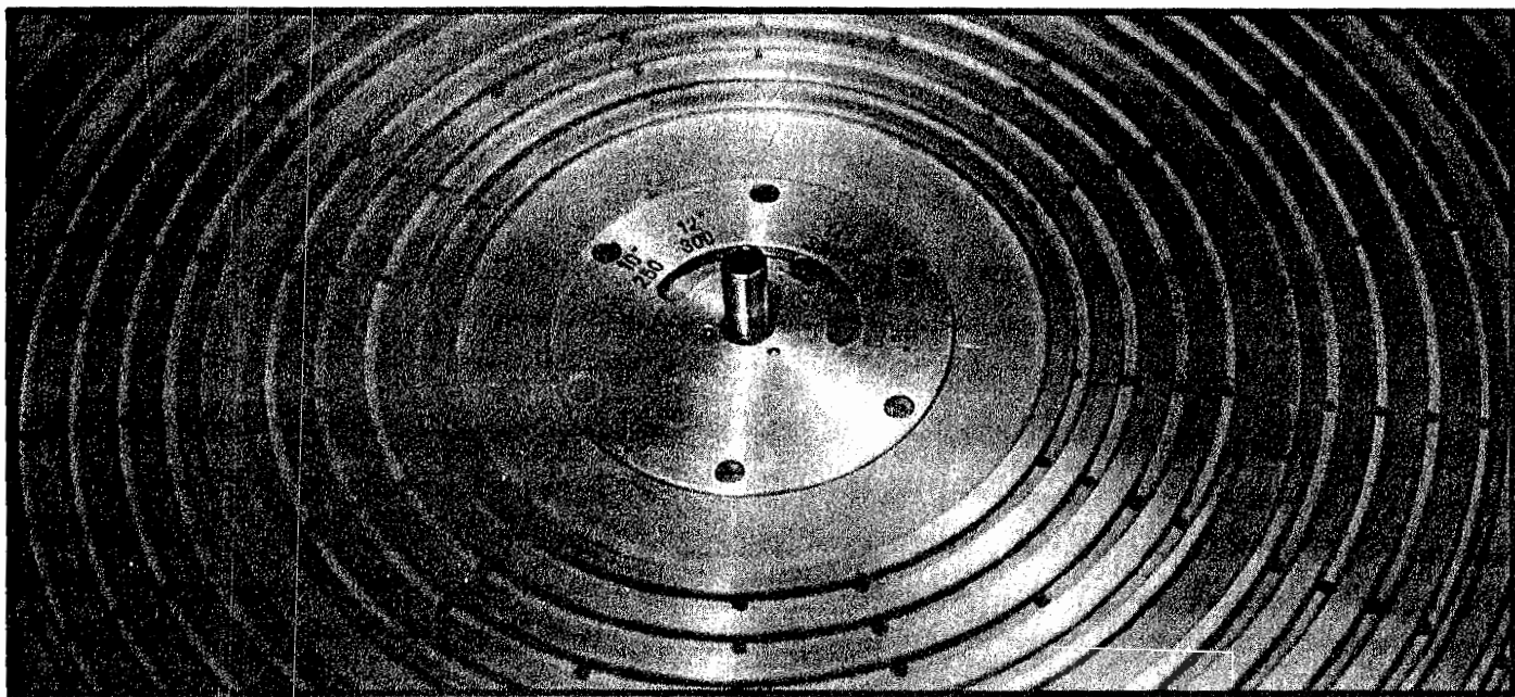
Close-up of the turntable of a Neumann Lathe, showing disc size selector and vacuum holes for disc hold-down.
