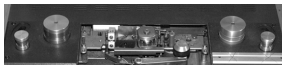
Figure 10: Modified A810 head assembly showing complete tape path with only the play head as a non-rotating element touching the tape surface.
