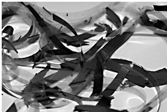
Figure 12: Binder-base adhesion failure in a Type III (Ferrochrome) cassette
