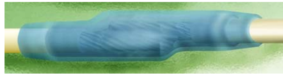
Figure 19-4. Double Sleeving over Soldered Connection
