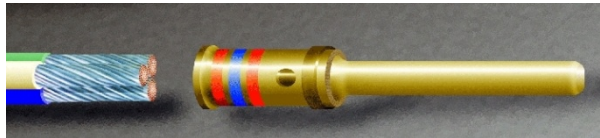
Figure 19-21. Stripped Wire Bundle Prior to Insertion
