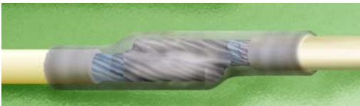
Figure 19-3. Sleeving over Soldered Connection
