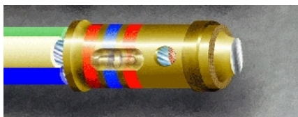
Figure 19-23. Contact Trimmed and Deburred
