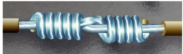
Figure 19-16. Completed Wrap for Western Union/Lineman Splice
